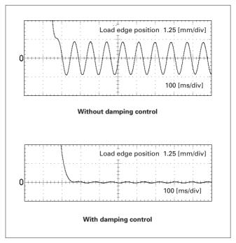
Fig. 6 Damping control characteristics
