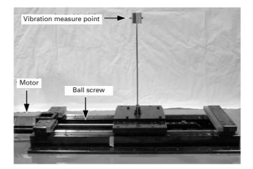
Fig. 5 Damping control evaluation machine
