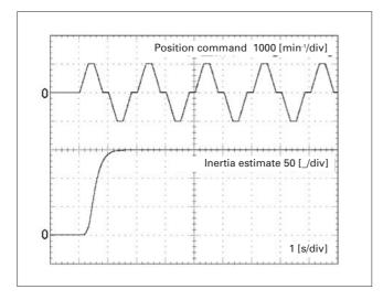
Fig. 2 Inertia estimation characteristics
