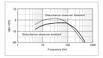
Fig. 4 Disturbance suppression characteristics
