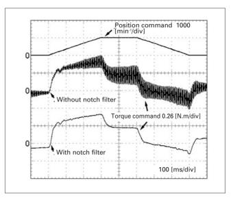
Fig. 3 High-frequency resonance suppression characteristics
